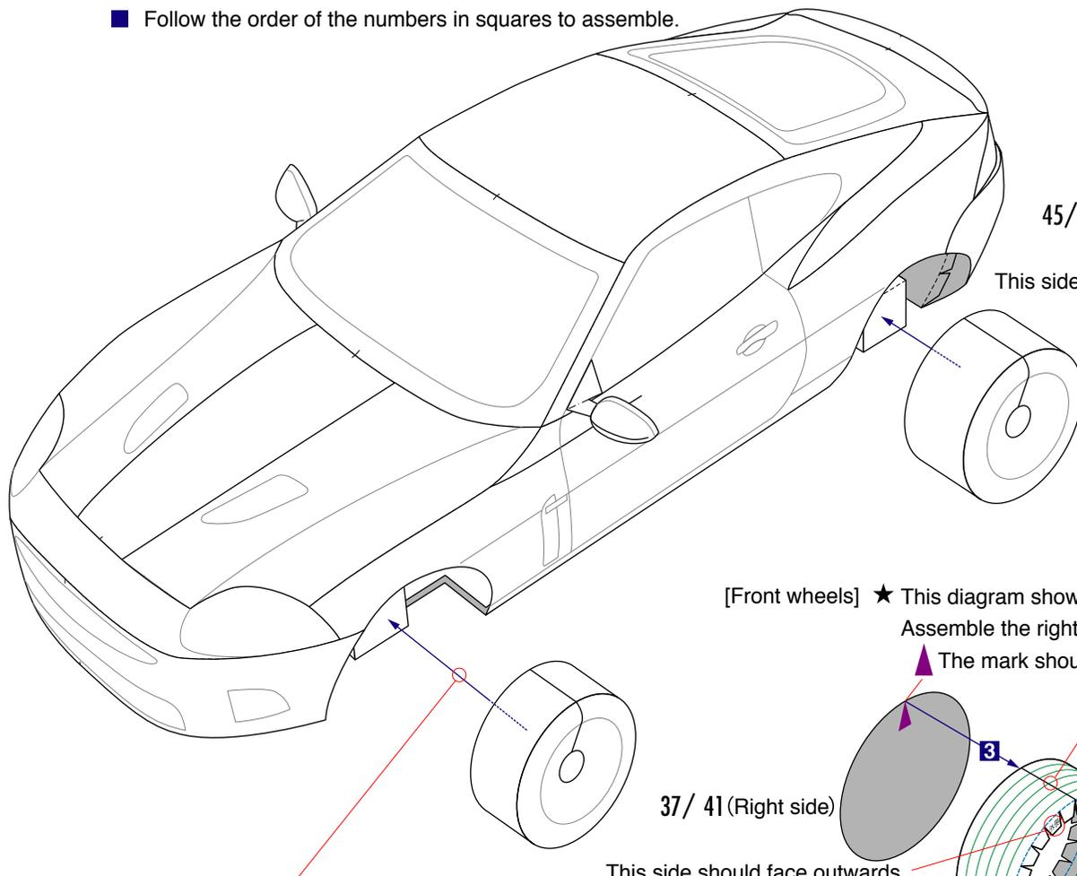
Look carefully at the gap between the wheel and the body of the car, ensuring that the left and right wheels are in line when they are attached.
